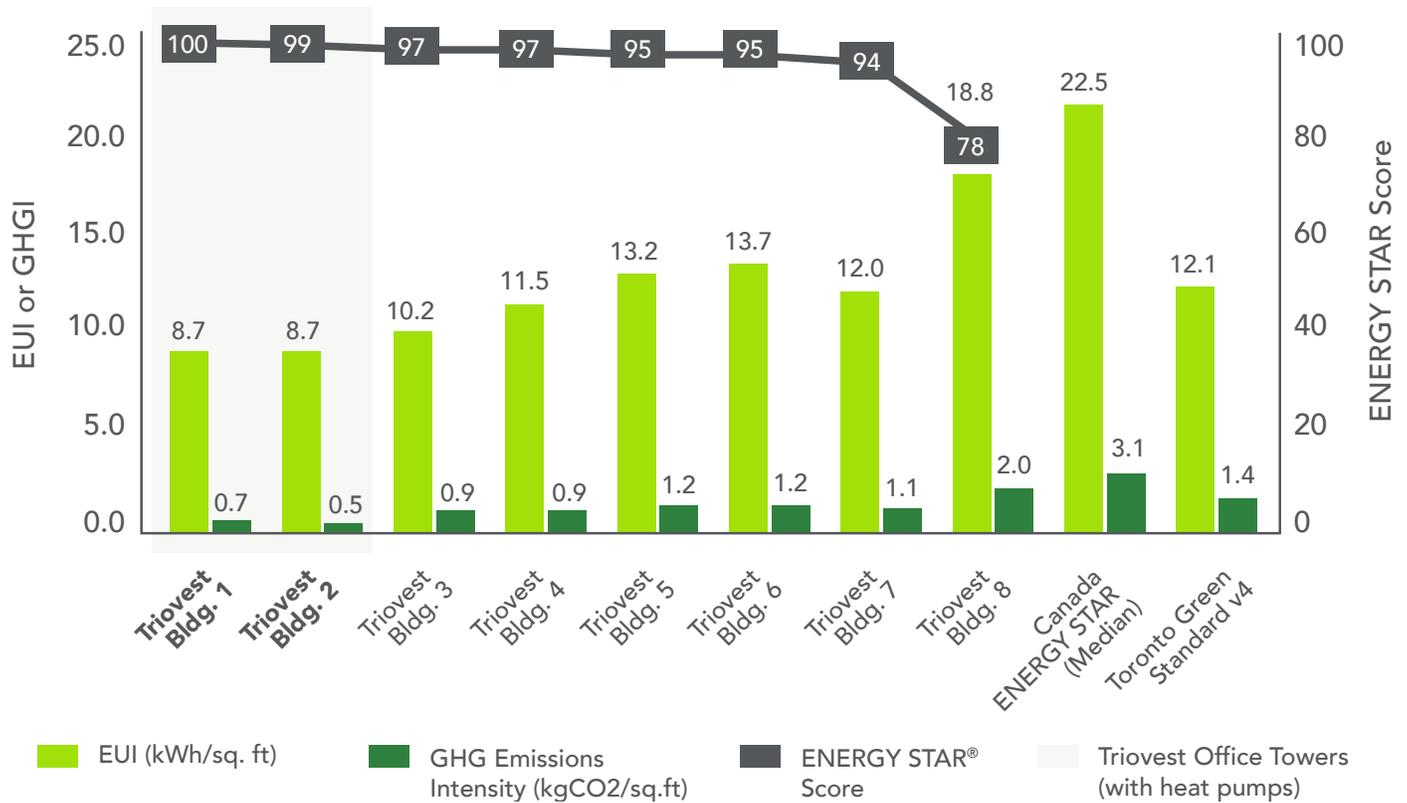
This graph compares the Energy Use Intensity (EUI) and Greenhouse Gas Intensity (GHGI) of the two Triovest office buildings with heat pumps to six other buildings in Triovest's portfolio. The graph also includes the [ENERGY STAR](#) median values for all benchmarked office buildings in Canada, and the [Toronto Green Standard](#) target for newly constructed commercial buildings.
